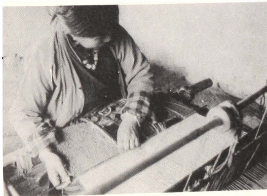
fig. 61 Making a looped carpet: cutting the loops.
