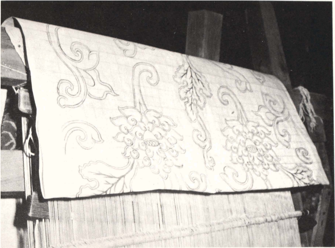
fig. 52 A carpet design drawn out on squared paper and laid over the top of the loom at the Tashi Jong Tibetan Settlement, Palampur.
