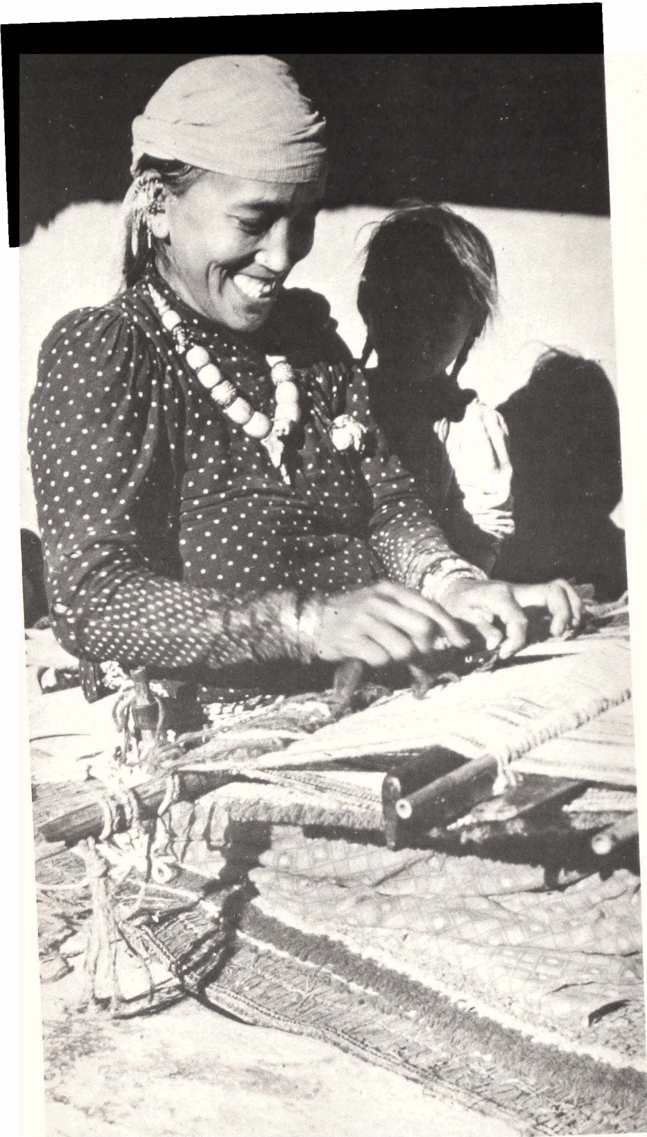
fig. 62 Making a looped carpet on the backstrap loom. The loops are being made round the gauge-rod. The weaver is a woman of the Thakali people of Nepal, but the same technique is used by Tibetans. She herself sits on a looped carpet.
