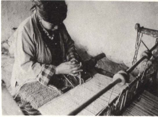
fig. 58 Making a looped carpet: the weaver is inserting lengths of pile yarn through the shed.
