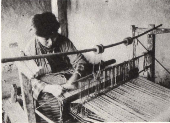
fig. 59 Making a looped carpet: making the loops round the gauge-rod.
