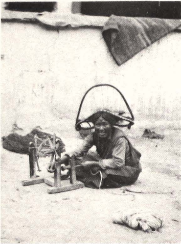
fig. 20 Reeling or playing yarn on a type of wheel also used for spinning (Drongtse 1933).
